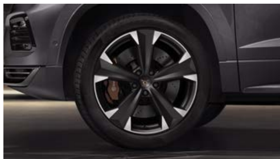
19" 'Sport' machined alloy wheels (optional performance brakes with front Brembo callipers shown)
